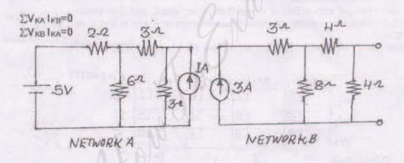
Where V<sub>KA</sub> and I<sub>KA</sub> are voltage and current in Network A respectively and V<sub>KB</sub> and I<sub>KB</sub> are voltage and current in Network B respectively.
